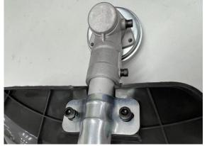
**Warning!** For brushcutter and grass trimmer operation, never use the machine without the guard assembled!
