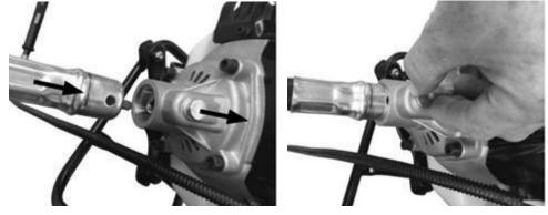
• Unscrew the air filter cover, screw the accelerator cable in as shown.
